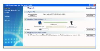
The Easy Upgrade Utility allows you to transfer system software, DDs, and HART device configurations between the 475 Field Communicator and a PC.
