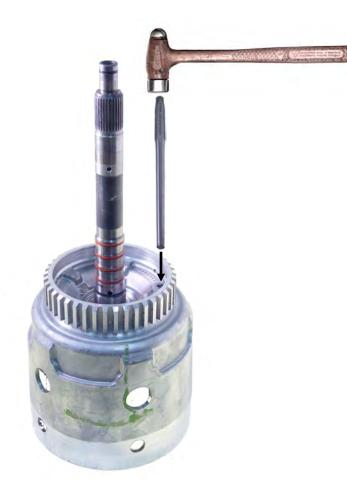
After orifice is installed 3-4 piston should not rock when placed in drum.
