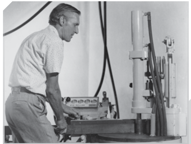
Reg Dobinson demonstrating his new invention, the 'Leaf Spring Eye Roller' 1977
