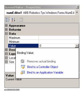
MenuDescriptionRemove actual bindingRemoves the existing data bindingBind to a Controller objectSelect available data in the controller for binding.Bind to an Application variableSelect available data in project temporary data store for binding.
