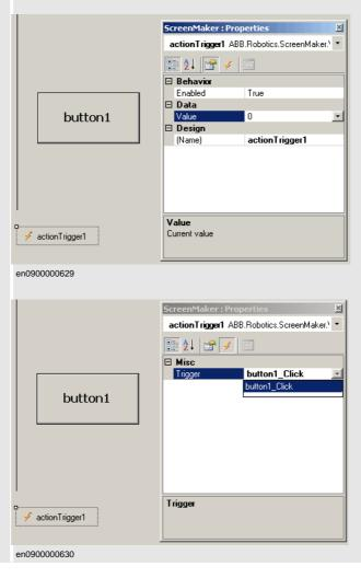
**NOTE:** An action is not triggered when the screen is launched for the first time, but is triggered when there is a difference in the binded value at any point of time. This functionality is supported only in RobotWare 5.12.02.
