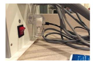
2) The vacuum hose needs to be inserted into the back of the machine with the gold prong with the outer blacklining.
