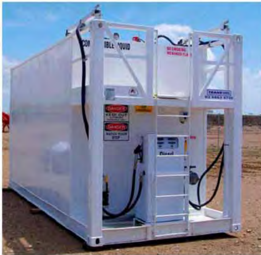
Figure 15 Internally Bunded Fuel Tank (Courtesy Transtank)
