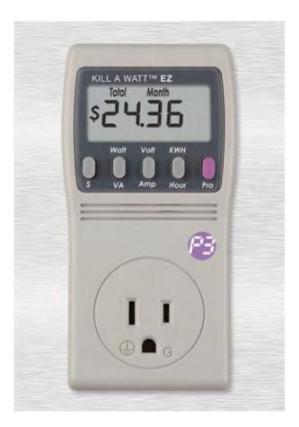
Then, I measured electric consumption of all pluggable electric devices in the house and put all sleeping electronic devices on switches. I replaced a 300 W halogen floor lamp by a 13 W compact fluorescent bulb, etc. This measures have reduced the baseload electric consumption by about 30%. All lights in the house are fluorescent and LED.
