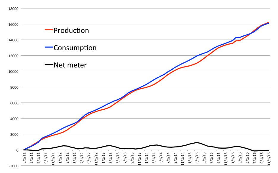
Annual PV 2.87 MWh, usage 2.5 MWh now vs. 6 MWh in 2010, typical home 14 MWh
