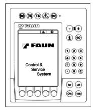
• After the system has passed through the system test without errors, the crane data display appears.
