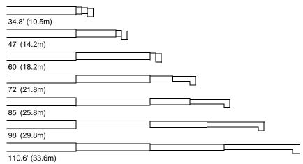
NOTE: Load radiuses for jib operation are given for reference with the boom fully extended to 110.6' (33.7m).
