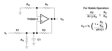
Figure 51. Non-Inverting CFB Integrator
