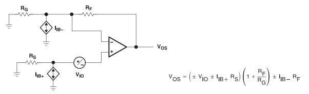
Figure 40. Output Offset Voltage Model
