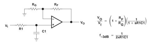
Figure 48. Single-Pole Low-Pass Filter
