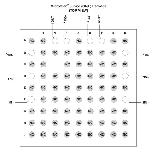
NOTE: Shaded terminals are used for thermal connection to the ground plane.
