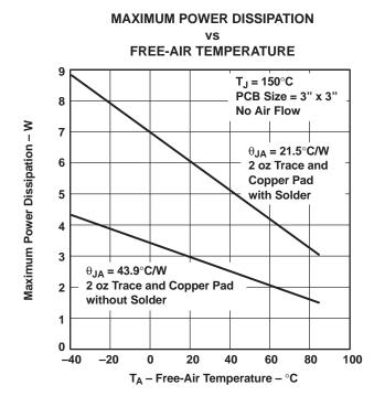
Figure 46. Maximum Power Dissipation vs Free-Air Temperature
