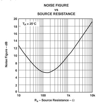
Figure 42. Noise Figure vs Source Resistance
