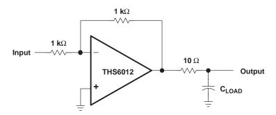
Figure 43. Driving a Capacitive Load
