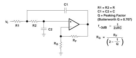
Figure 49. 2-Pole Low-Pass Sallen-Key Filter
