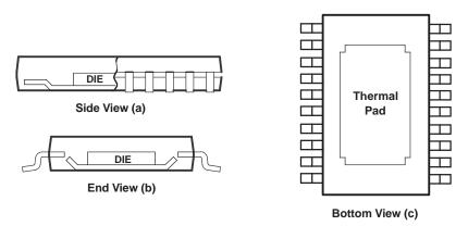
A. The thermal pad is electrically isolated from all terminals in the package.
