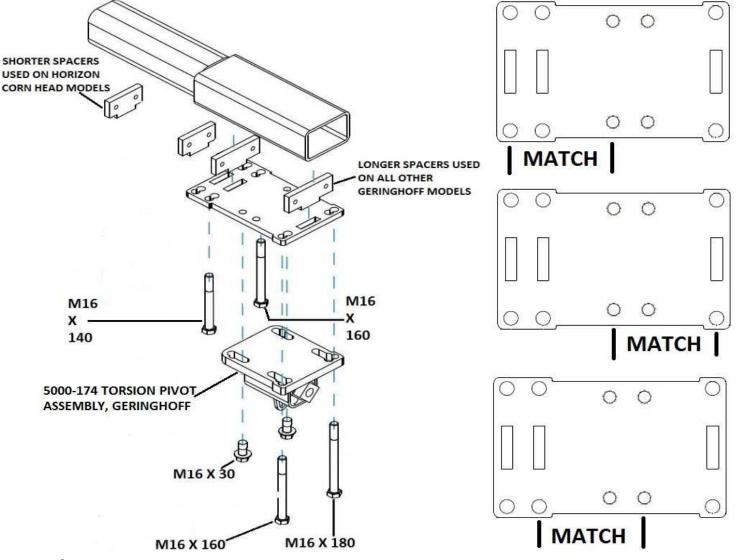
BELOW ARE RECOMMENDED LOCATIONS OF THE TORSION PIVOT ASSEMBLY, ALTERNATE LOCATIONS MAY BE USED IF INTERFERENCE OCCURS!
