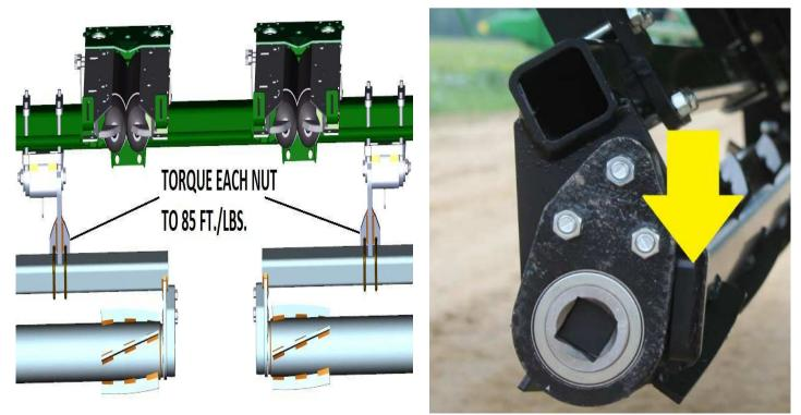
**Step 4:** Install the Devastator roller, spacer/bushing and bearings to the roller tube using the  $\frac{1}{2}$ " x 2-1/2" carriage bolts. A 3R30 roller is pictured in the diagram below. <u>IMPORTANT</u>: The spacer must be installed between the roller and the bearing. The notches of the bearing housing must face the mounting plate. The extended race on the bearing will face away from the roller.
