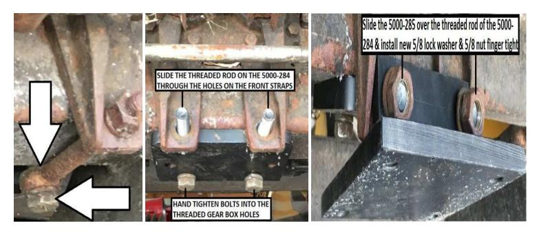
**Step 2**: Place the 5000-167 torsion pivot assembly on the 5000-285 adaptor aligning all 4 holes. Thread by hand the 2502-810 M16 X 2 X 30 bolts on the front set of holes. Place the spacer between the 5000-284 calmer adaptor bracket & the 5000-285 adaptor. Thread by hand the 2502-809 M16 X 2 65 bolts. Tighten the hardware from steps 1 & 2 to torque spec in the following order:  $A - 1^{st}$ ,  $B - 2^{nd}$ ,  $C - 3^{rd}$ ,  $D - 4^{th}$ .
