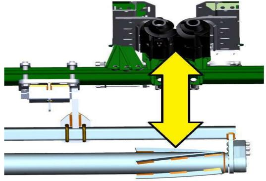
**Step 6: (If Applicable)** On chopping corn heads, trim 3 inches off the bottom of the back curtain to keep the roller from contacting the curtain.
