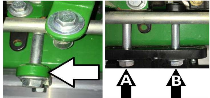
**Step 2:** Install the 5000-292 Torsion Arm onto the Torsion Pivot Assembly & secure with the  $\frac{3}{4}$ " x 8" bolts &  $\frac{3}{4}$ " lock nuts. Refer to the diagrams on the pages  $\frac{10 - 12}{10}$  to determine which side of the Torsion Pivot Assembly to install the 5000-292 Torsion Arm.
