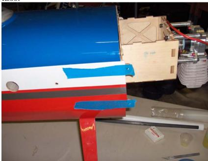
28. Place the canopy/hatch onto the fuselage to aid in alignment. Peel the tape back just behind the F1 former and place the cowl into position. You will need to open the cowl to clear the cylinder head of the engine. Place your spinner (4 inch) on the motor to help align with cowl. View the cowl from several angles to insure that it is positioned properly. When satisfied put the four tape strips back into position and drill a 1/8" hole at the location of each of the 4 ink marks.
