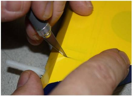
2. Insert the 2 control horns into the base plate and trial fit the horns into the slot and make sure they seat properly against the base and elevator surface. Trace around the
