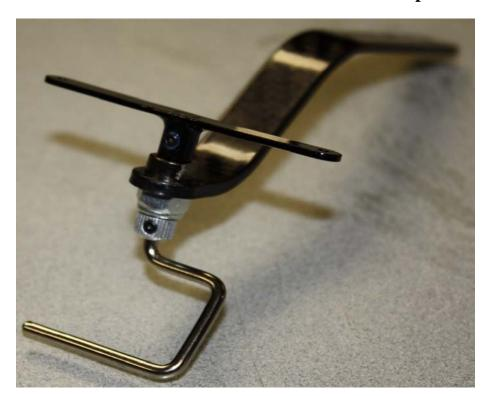
20. Place the tailwheel assembly on the rear bottom of the fuselage and secure with a piece of tape. Drill holes at the location of the mounting holes and secure the tailwheel bracket with the included course thread wood screws.
