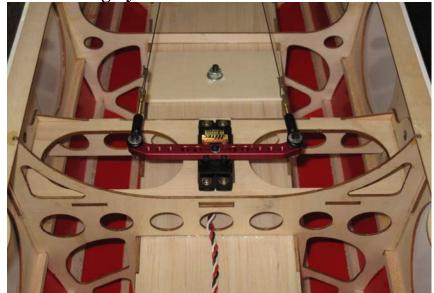
We are using the SWB 4" offset rudder arm. We highly recommend the use of this quality product to ensure correct geometry.
