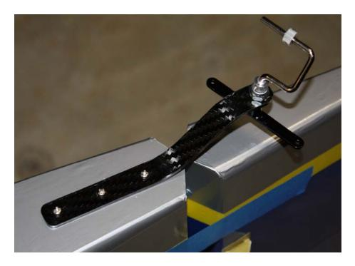
21. Mount the tiller arm as shown and insert the ends of the springs into the holes in the ends of the arms and bend to secure.
