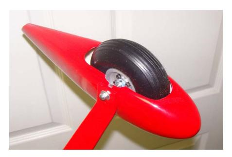
17. When satisfied with the position of the wheel pants, drill a hole though the plywood plate that is glued inside the pant at the location of the hole in the landing gear. Secure the pant in position with the provided 3mm bolt and blind nut. Repeat this process for the remaining wheel pant.
