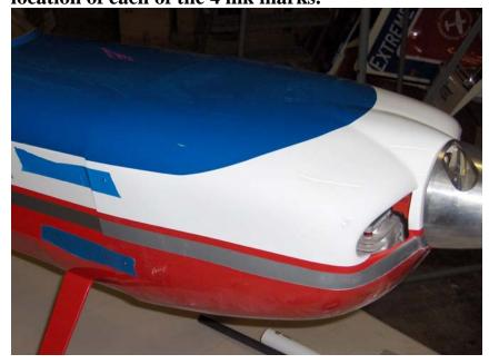
29. Secure the cowl using 4 3mm socket head bolts in conjunction with 4 bonded sealing washers as shown.
