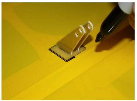
11. Locate the aileron servo mount and remove the covering from this area. Use a sealing iron to seal the edges of the covering to the sides of the servo opening. Take a few minutes to apply some CA to the joints of the servo rails and the ribs.
