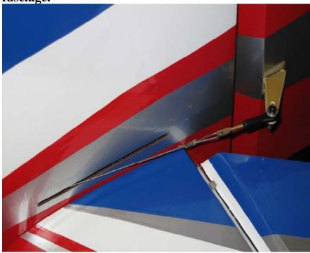
25. Assemble one end of the linkage by inserting the pull-pull cable into one of the aluminum tubes, through the hole in the brass pull-pull fitting and back through the aluminum crimp tube. Loop the cable back through the crimp tube a second time and crimp with side cutters.
