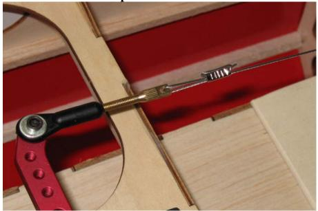
26. Insert the bare end of the cable into the slot in the rear of the fuselage and feed it forward into the canopy area and make up the same type of linkage as you did previously. Electronically center your servo. Secure the linkage at both ends with a 3mm bolt and nylon insert lock nut. Repeat for the other side. Pull-pull cables should be <u>crossed</u> for this installation on the Edge.
