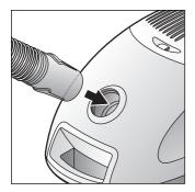
Push the flexible tube adapter into the air intake opening in the vacuum cleaner lid until it engages
