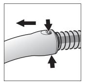
The handle can easily be detached from the hose to remove blockages.
