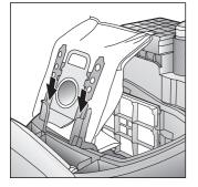
Slide the new dust bag into the holder to the stop.
