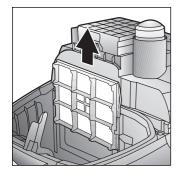
Pull out the motor protection filter in the direction of the arrow.
