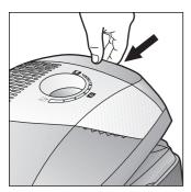
Open the lid by moving the locking lever in the direction of the arrow.
