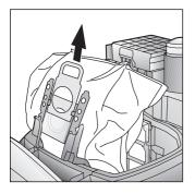
Seal the dust bag by pulling the sealing strip and remove the bag.
