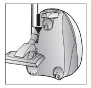
To store/ transport the vacuum cleaner, use the storage aid on the underside of the vacuum cleaner.
