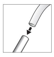
Connect together the handle and telescopic tube.
