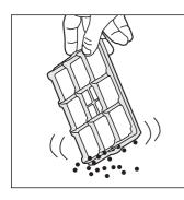
Clean the motor protection filter by tapping it.
