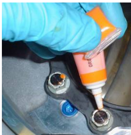
Figure 2 - Correct Application of Torque Seal
