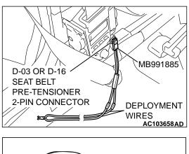
6. Connect the D-03 or D-16 seat belt pre-tensioner two-pin connector to special tool MB686560 and move the deployment wires out of the vehicle.
