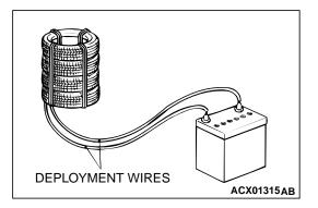
6. Place three old tires without wheels on top of the tire secured to the air bag module, and secure all tires together with ropes (four locations).
