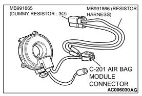
(3) Connect special tool MB991865 to special tool MB991866.
