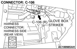
STEP 3. Check the harness wires for short circuit to ground between SRS-ECU connector C-12 (terminal No.9 and 10) and passenger's air bag module connector C-106 (terminal No.1 and 2).
