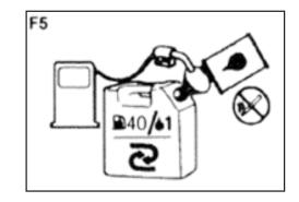
Most engine troubles are caused, directly or indirectly, by the fuel used on the machine. Take special care not to mix a motor oil for 4-cycle engines.
