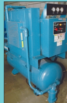
15 HP Quincy Model OST15ANA32SS Rotary Screw Horizontal Tank Air Compressor
