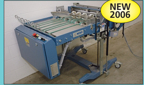
MBO Model ASP66-1ME Mobile Stream Delivery Machine w/ Splitting Device & Pressing Integrated Marking Device
