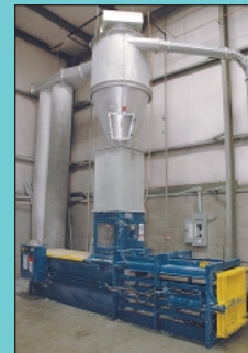
Balemaster Balewell Open End Horizontal Hydraulic Baler w/ Shredder
