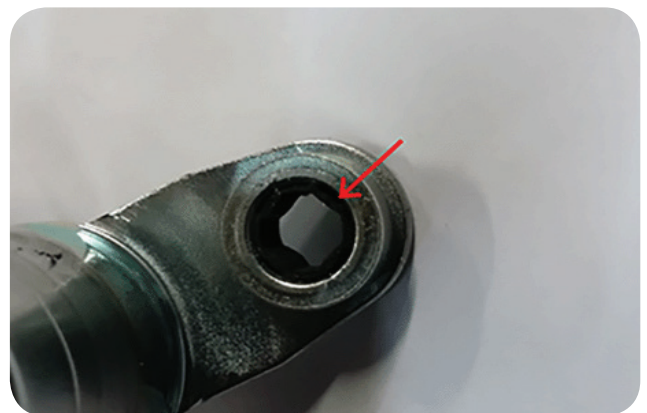
Black plastic bolt retainer in the solenoid hold down ear
