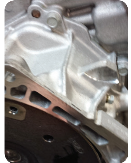
Routing the strap over the sharp bell housing edge may cause it to be cut and break.
