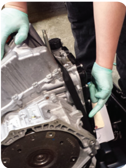
Place the strap around the side of the bell housing, not over the sharp front edge.
