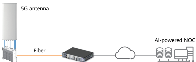
Figure 5-5 System diagram of a 5G network
