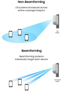
Figure 3: Traditional antenna radiation vs. Beamforming
