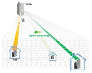
Figure 4: Beam switching
