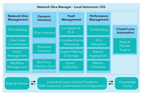
Figure 9: Functional Architecture - Local Autonomic OSS
