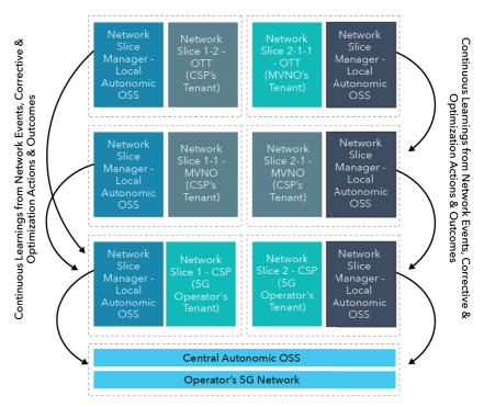
Figure 7: Recursive OSS Systems for 5G Network Operations
