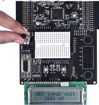
Figure 5-3. Voltage Display using SAR ADC
