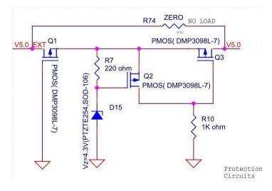
Figure 4-8. Schematic for Protection Circuit on 5-V Power Line
