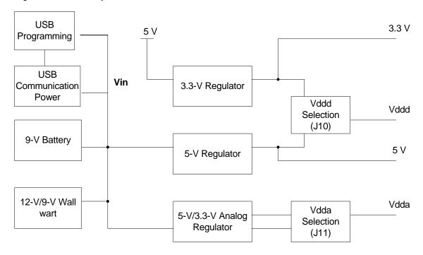
Figure 4-2. Power System Structure
