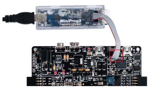
With the MiniProg3, programming is similar to the on-board programmer; however, the setup enumerates as a MiniProg3.
