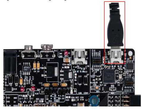
When the USB programming is plugged into the PC, it enumerates as DVKProg5 and you can use the normal programming interface from PSoC Creator to program this board through the on-board programmer.
