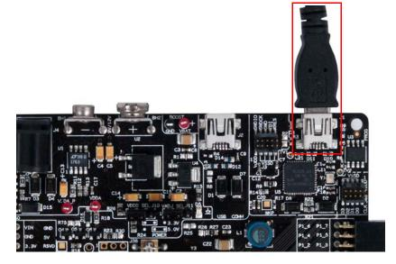
When plugged in, the board enumerates as DVKProg5. After enumeration, initiate, build, and then program using PSoC Creator.
