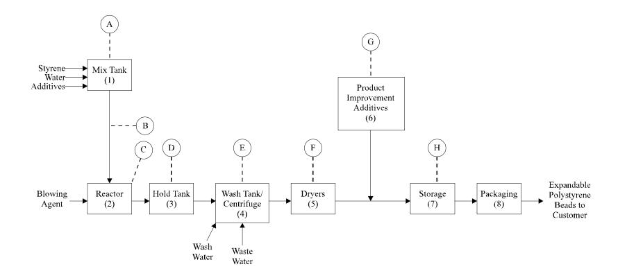
Figure 6.6.3-4. Simplified flow diagram of the expandable polystyrene in-situ suspension process.
