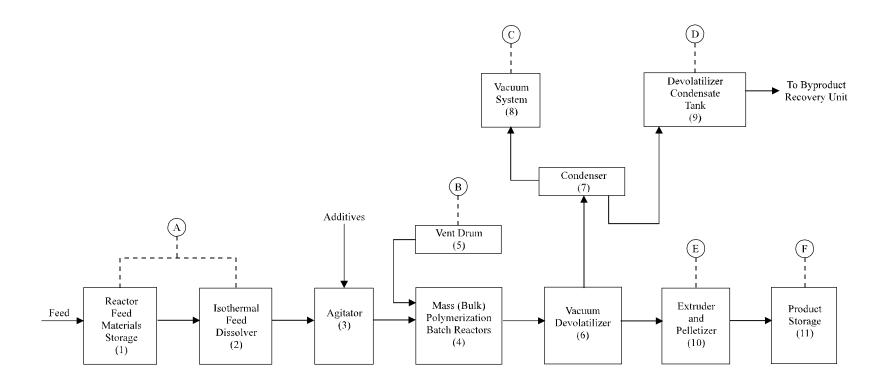
Figure 6.6.3-1. Simplified flow diagram of a batch polystyrene process.
