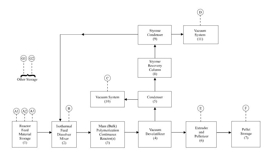
Figure 6.6.3-2. Simplified flow diagram of a continuous polystyrene process.
