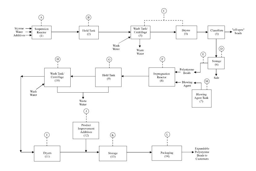
Figure 6.6.3-3. Simplified flow diagram of the expandable polystyrene post-impregnation suspension process.
