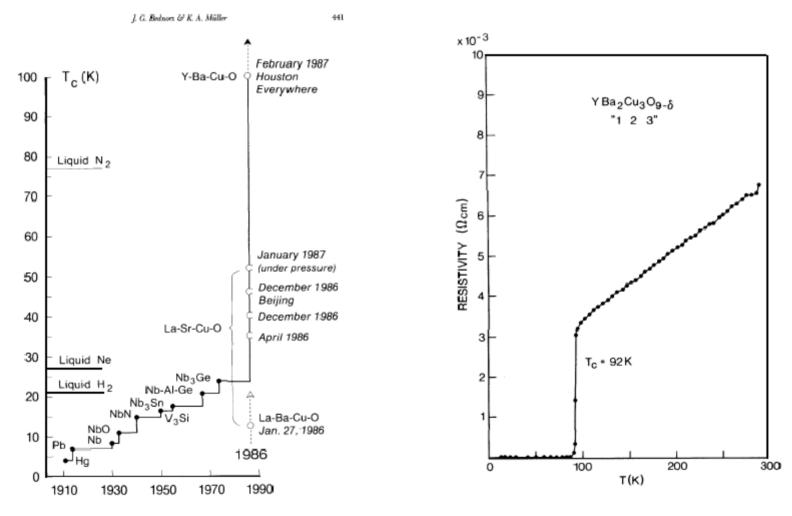
Figure 1.13. Evolution of the superconductive transition temperature subsequent to the discovery of the phenomenon. From [1.29], (2) 1987 by the American Association for the Advancement of Science. Figure 2.24 Resistivity of a single-phase YBagCu3O3 sample as a function of temperature.
