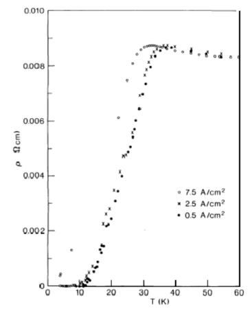
Figure 1.5. Low-temperature resistivity of a sample with x(Ba) = 0.75, recorded for different current densities. From [1.19], © Springer-Verlag 1986.
