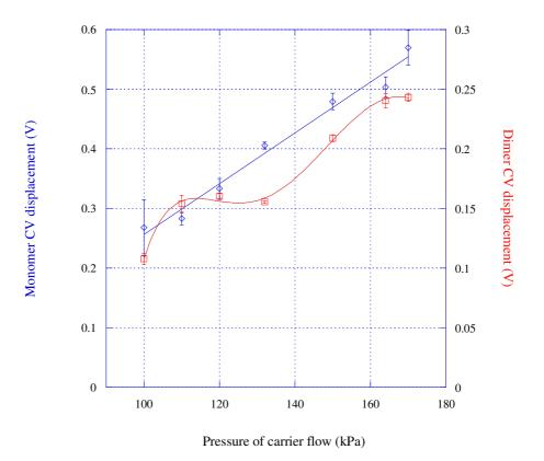
**Figure 6.10** Compensation voltages of peak response of Ethyl Acetate from the GC-FAIMS system over a range of pressures. Monomer (blue diamonds) and dimer (red squares) responses are displayed alongside one another. System maintained at a constant E/N.
