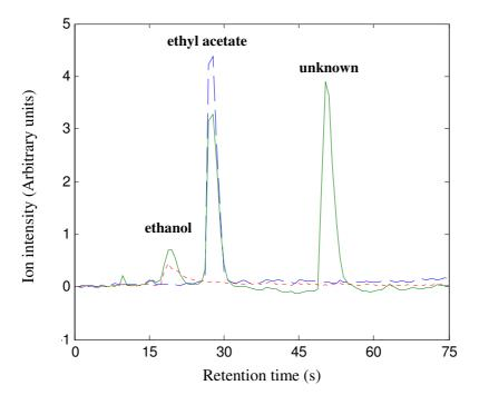
Figure 6.7 Signal isolated at peak response of ethyl acetate for solutions of ethyl acetate in distilled water (blue dashed), ethanol in distilled water (red dashed) and wine (green solid). Labels are the inferred compounds responsible for the signal.
