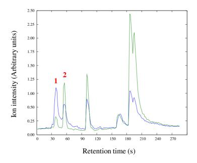
**Figure 6.3** Two plots of ion response versus retention time at specific CV values of a full GC-FAIMS response are shown. The CV values isolated were selected as being characteristic of the peak ion response of the first peak (blue) and second peak (green).
