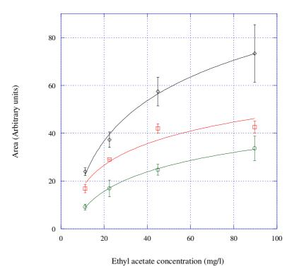
**Figure 6.16** The response from ethyl acetate at various concentrations; at a carrier flow pressure of 122 kPa in distilled water (black diamonds), solvent of ethanol (12%) in distilled water (red squares) and at an ambient carrier flow pressure in a solvent of distilled water (green circles).
