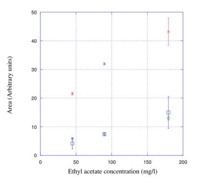
Figure 6.8 Ethyl acetate spiked solutions with various solvents; Distilled water (red), distilled water and 12% ethanol (blue) and wine (green).
