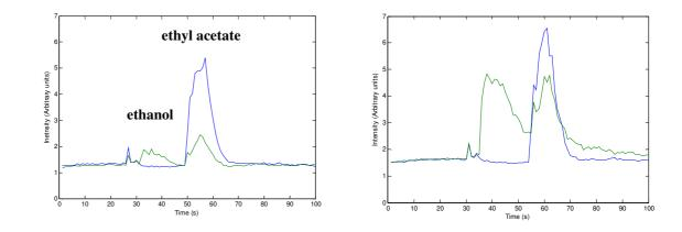
**Figure 6.12** Responses obtained from the GC-FAIMS system at a gauge pressure of a) 120 kPa and b) 136 kPa. Ethyl acetate in solvents of distilled water (blue) and distilled water and 12% ethanol (green) are shown alongside one another.
