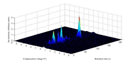
Figure 6.2 Surface plot of data obtained over 267 seconds from a 0.5  $\mu$ l injection of wine into the GC-FAIMS system in the positive mode.
