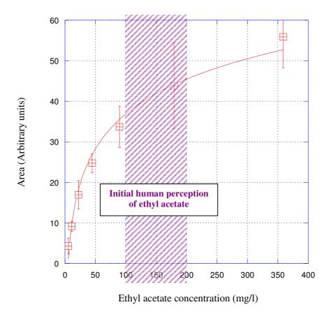
Figure 6.4 The response obtained in the GC-FAIMS system from spiked samples of distilled water with various concentrations of ethyl acetate.
