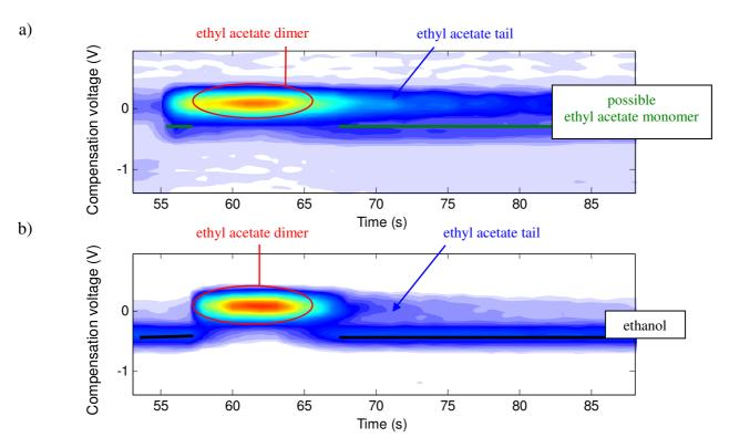
**Figure 6.14** Reponses obtained from the GC-FAIMS system operating with an ambient pressure of carrier flow to FAIMS unit. a) Injection of distilled water spiked with ethyl acetate b) Injection of ethyl acetate within a solvent of distilled water and ethanol (12%).
