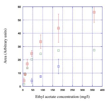
**Figure 6.9** The response obtained for ethyl acetate within distilled water (red), and wine (blue + green). The red and blue data was obtained with a non-polar column and the green data was obtained with a polar column.
