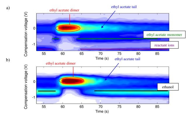
**Figure 6.15** Reponses obtained from the GC-FAIMS system operating with a carrier flow pressure of 177 kPa (absolute) to the FAIMS unit. a) Injection of distilled water spiked with ethyl acetate b) Injection of ethyl acetate within a solvent of distilled water and ethanol (12%).
