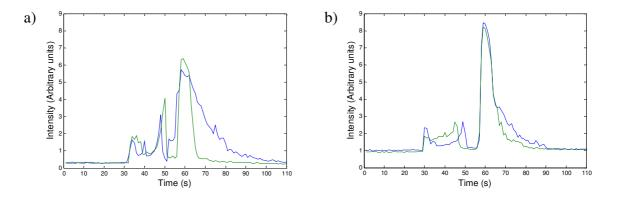
**Figure 6.13** Responses obtained for high concentrations of ethyl acetate within distilled water (blue) and a solvent of distilled water and 12% ethanol (green), a) was undertaken with a carrier flow at ambient while b) used a carrier flow of 177 kPa.
