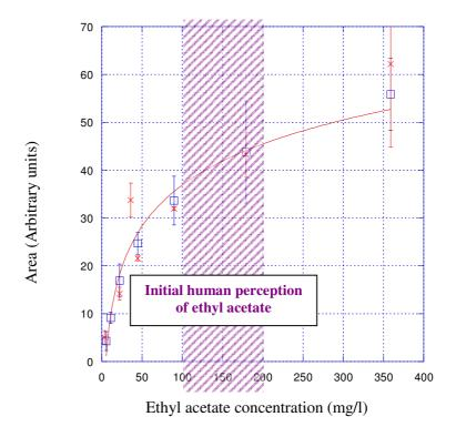
**Figure 6.5** Responses obtained from samples of distilled water spiked with various concentrations of ethyl acetate from investigations undertaken two weeks apart (blue squares and red crosses).
