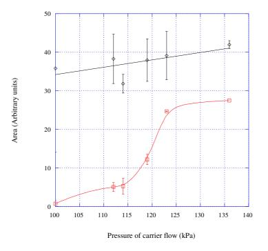
Figure 6.11 Area of ion response of ethyl acetate from a solvent of distilled water (black) and distilled water and 12% ethanol (red).
