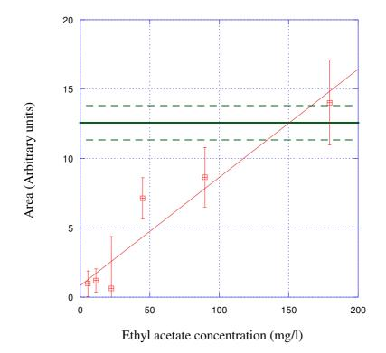
**Figure 6.6** The response obtained in the GC-FAIMS system from samples of wine spiked with different concentrations of ethyl acetate minus the response from un-spiked wine (red crossed squares). The average response (solid green) and limits from a single deviation of triplicate readings (dashed green) from un-spiked wine is also given.
