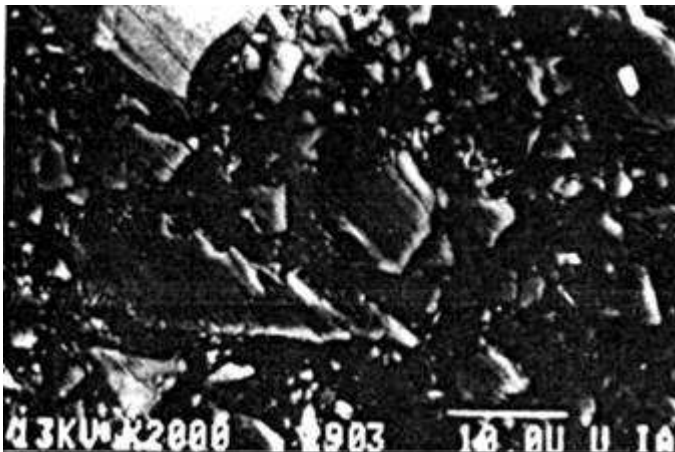
FIGURE 41.4 Microstructure of a dental composite. Miradapt o (Iobnson & Iohnsonj) 50% by volume filler: barium glass and colloidal silica [Park and Lakes, 1992].
