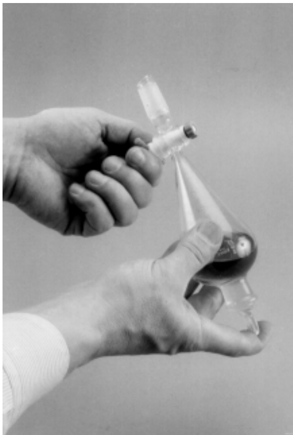
Figure 6.6: The proper method to vent a separatory funnel.
