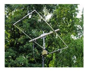
approximately 9 % larger (or smaller) than the active element. If larger, it acts as a reflector, and if smaller, a director. It is easy to feed, as it is simply a dipole with a parasitic element mounted nearby. A Moxon beam has a smaller footprint than some other beam designs, while providing nearly the same gain and front-to-back ratio, as a typical two-element Yagi beam.
