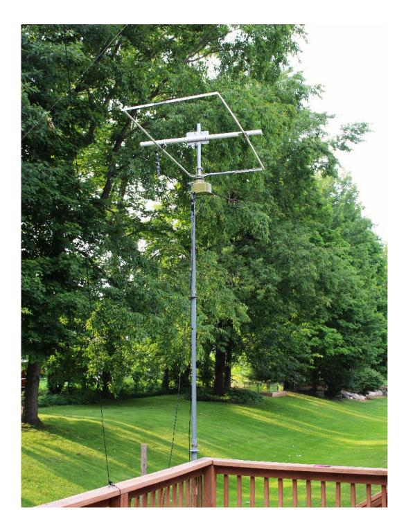
I tuned it at this height. The deck railing is approximately 9 feet above the turf. Ultimately, I will raise it another ten feet after I finish tuning and pruning it.
