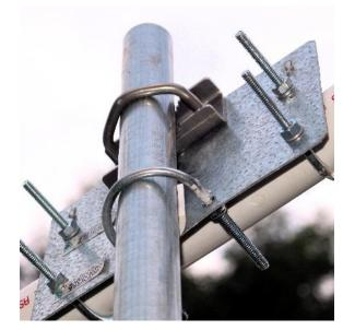
I used an inexpensive RCA TV rotator and a 1.5 foot long section of 1.25 inch diameter galvanized television antenna mast I had on hand. It was just long enough to raise the antenna above the rotator, but not allow too much torque in case of strong wind.
