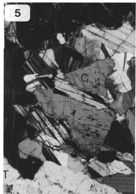
Plate 2. Examples of microstructures in weakly and moderately recrystallized textures (crossed polarized light). 1. Weakly recrystallized plagioclase and olivine. Rotation recrystallization is evident in plagioclase where subgrains rotate deformation twins (s). Recrystallized plagioclase grain boundaries commonly meet at 120^\circ triple points. Neoblast boundaries are generally smooth and gently curved. The igneous morphologies of olivine grains are still evident, but some polygonization occurs on the grain extremities. Sample 153-921D-5R-2, 68–73 cm. 2. Plagioclase neoblasts in a weakly recrystallized gabbro. Albite and perthite deformation twins tend to be more abundant in the moderately recrystallized texture, but the neoblast characteristics are otherwise similar. Sample 153-923A-8R-2, 13–19 cm. 3. Relict plagioclase grain in moderately recrystallized texture displaying complex substructure. The margin of the relict grain is highly irregular. Deformation twins (T) within the grain are deformed by bending of the crystal lattice as indicated by the patchy undulose extinction. Subgrain (S) formation rotates the deformation twins by less than 5^\circ . Some of the recrystallized grains have small, isolated protrusions at their margins, suggesting that limited grain boundary migration occurred. Sample 153-923A-3R-1, 100–105 cm. 4. Kink band in relict plagioclase grain in weakly recrystallized texture. Albite deformation twins are deformed by the sharp boundaries of a 0.5-mm-wide kink band. Sample 153-923A-8R-2, 81–88 cm. 5. Undeformed clinopyroxene oikocryst containing plagioclase inclusion. The dismemberment of clinopyroxene (C) oikocrysts can be traced from their primary igneous textures to partial disruption (as in this example) and to complete separation where the plagioclase matrix and inclusions are indistinguishable and dismembered clinopyroxene crystals with characteristically straight edges are suspended in the plagioclase matrix. This process gives many samples a brecciated appearance, although the separation of clinopyroxene fragments may be a dominantly crystal-plastic process. Sample 153-922A-2R-5, 68–73 cm.
