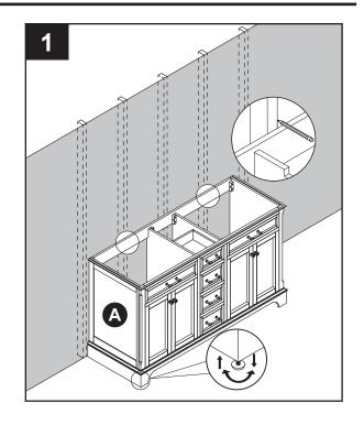
2. Using hardware appropriate for your wall type (not included), secure vanity cabinet (A) to two wall studs anywhere through the vanity mounting plates. Be careful not to disturb any electrical or water lines that may be concealed in the wall.
