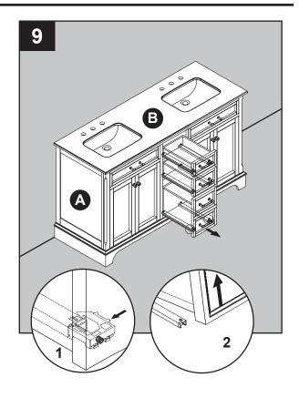
10. To re-install drawers into vanity (A). Please fully extend metal glide tracks, gently lower and slide drawer box into rear glide catch, then, lower drawer box down to completely rest on extended glides, push plastic levers to lock the drawer box in place.
