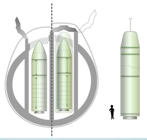
Left profile: the SNLE-NG (Le Triomphant type) with the present M45 missile; Right profile: M51 missile, with aerospike extended
