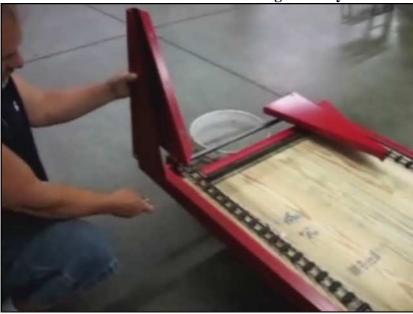
4. Assemble the front slant panel boards by bolting the 3 predrilled short boards to the left and right slant panels, using 6 - 1/4" x 1-1/2" carriage bolts and nuts.
