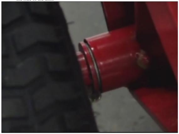
WARNING: The axles must be greased on a weekly basis, under regular use. This will prolong the life of the axles and bearings.
