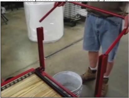
7. Mount 1 Beater support bearing using 2 - 5/16" x 2-1/4" bolt/nut/washer assemblies to the left side beater support.
