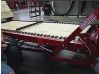
13. Loosen bolt on the backside of the clutch handle.
