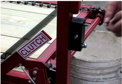
8. Slide short stub of beater into installed beater support bearing. Slide other beater support bearing onto long shaft side of beater and install on the right side, using
