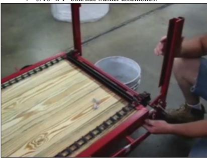
6. Insert beater stabilizer bar into the square tube on each beater support. Make sure tube is flush with the bottom of the square tubes. Slight hammer tapping might be necessary using a wood block between hammer and bar. Insure that the bar is not cocked to preclude binding of beater during operation.
