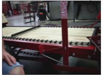
15. Loosen and slide forward the set collar on the clutch hold rod. Move collar 1/2" away from keyhole slot on the frame. Once set, disengage clutch to check belt
