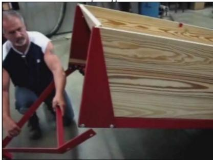
21. Remove the front bolts of the slant panel, and swing the tongue into place. Put the bolts in place and tighten everything with a wrench.
