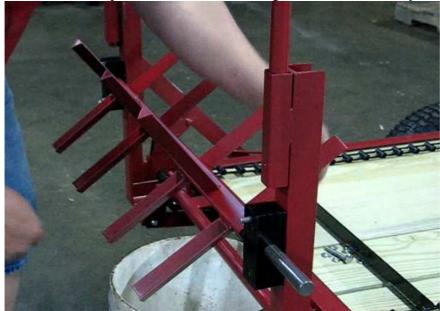
9. Install the 3/16" x 5/8" keyway into the beater shaft as shown. Tap keyway until full seated in slot.
