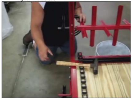
11. Install the v-belt as shown. Make sure the belt is under the belt tightener rod.
