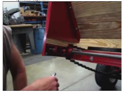
19. Ensure that the drag chain has 2 to 3 inches of sag under the load bed. Periodically check the chain tension, as the chain stretches over time.
