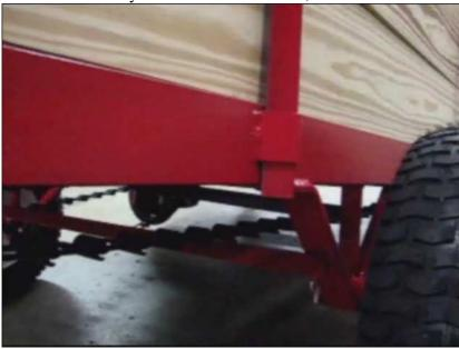
Remove the rear bolts in the front slat panel assembly to mount the tongue. Place the tongues rear holes over the slant panels holes, and hand tighten the bolts.NOTE: The tongue can be mounted at two different heights. Please determine what works best for your application.
