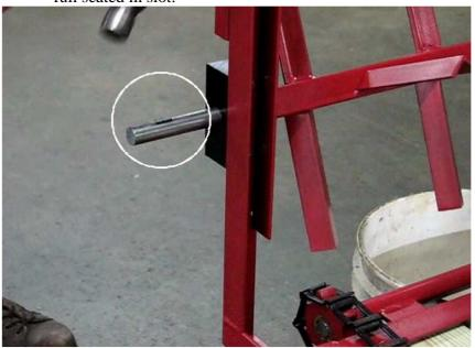
10. Install the beater shaft pulley on to the beater shaft with the set collar facing out. Make sure that the beater shaft pulley is in line with the lower dive pulley. Tighten allen screw.
