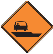
Low shoulder ahead. Difference in elevation due to construction
