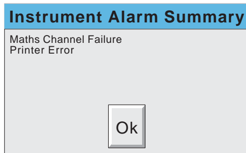
Figure 3.1.4b Typical Instrument alarm summary display
