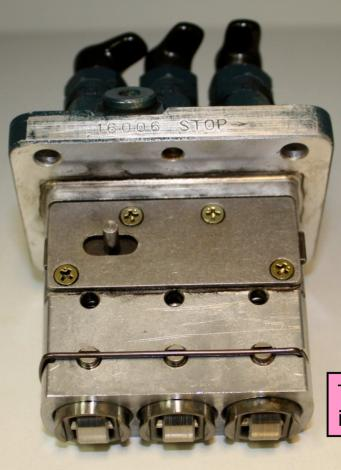
When the repair is complete the control lever should move form side to side when tilting the pump.
