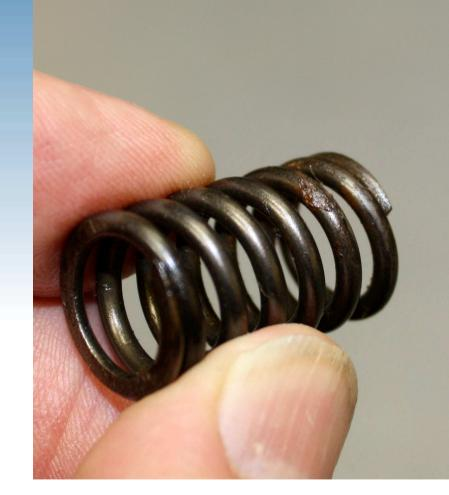
Spring : Kubota p/n 15841-51280 If there is rust the springs need to be changed. It is a good idea to change all 3 springs when doing this repair.
