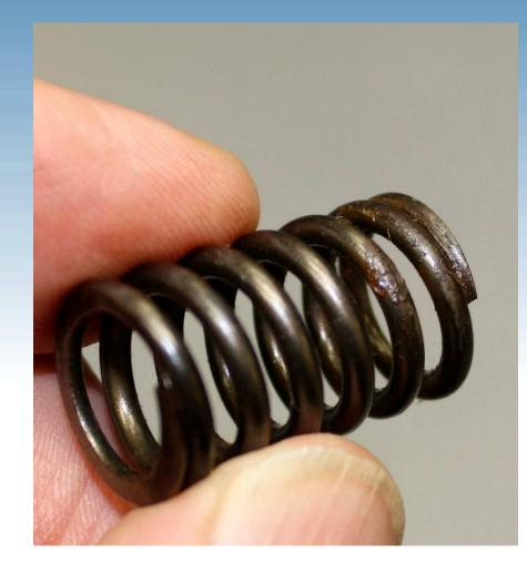
Spring : Kubota p/n 15841-51280 In this picture there is rust that will cause the spring to break soon.
