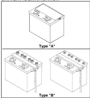
Compare the battery in your lawn tractor (located under the seat) with the illustration above. Type "A" batteries are activated and are ready to use. Type "B" batteries must be filled with battery fluid (acid) and charged before they are put into service. Follow the instructions which apply to the battery in your lawn tractor.
