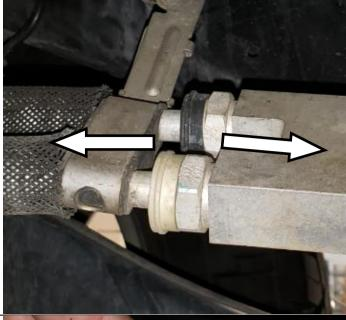
The original thermostat housing should now be removed. Clean the ends of the lines if needed to prevent debris contamination upon reassembly.
