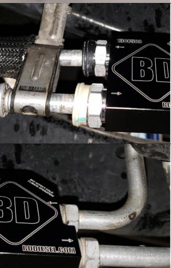
Inspect original O-ring on the tube, replace with supplied viton O-ring (1453153) if it is damaged.
