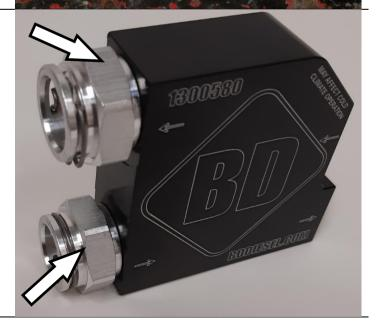
Lubricate the o-ring and clip using transmission lubricant
