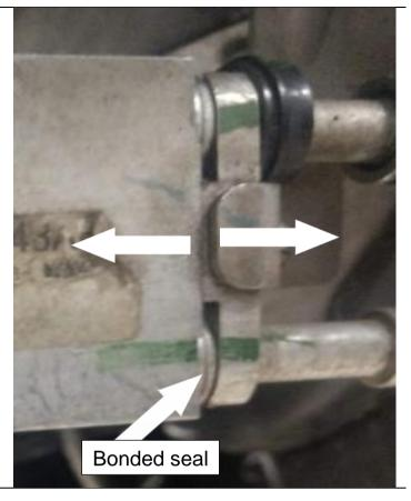
Inspect original O-ring on the tube, replace with supplied viton O-ring (1453153) if it damaged.
