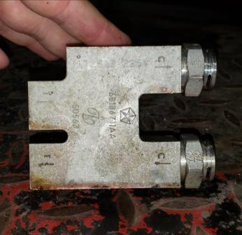
Put quick connect fitting (1300579) on thermal by pass block (1300580) using 1" and 24mm open wrench.
