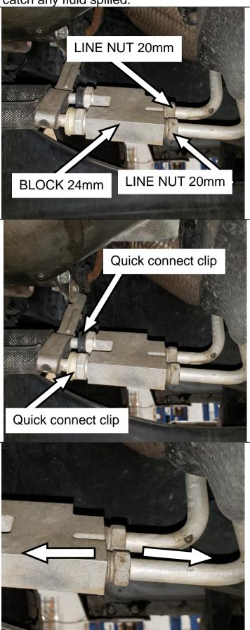
Pull cooler bypass block off of the quick connect lines
