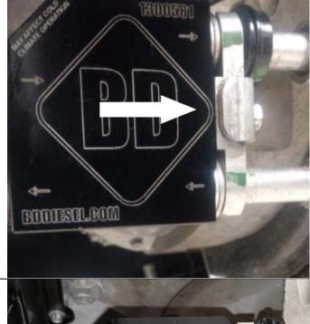
Reinstall both transmission cooler lines in to threaded end of the block, wiggle the lines and nut to start the threads. Tighten nuts 24 lb-ft.
