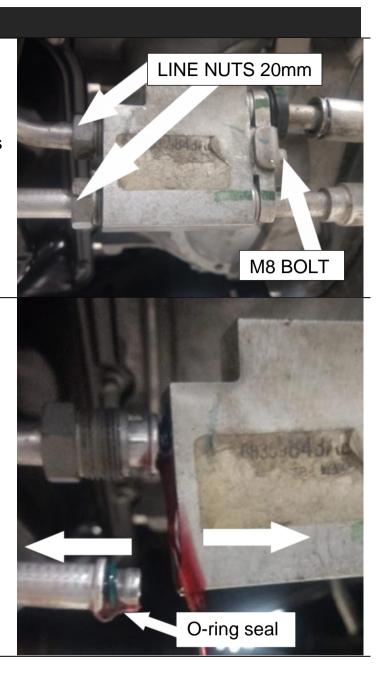
Pull the cooler bypass block off of the bracket to disconnect the lines
