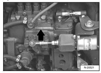
The engine serial number is in the location shown [Figure 3].
