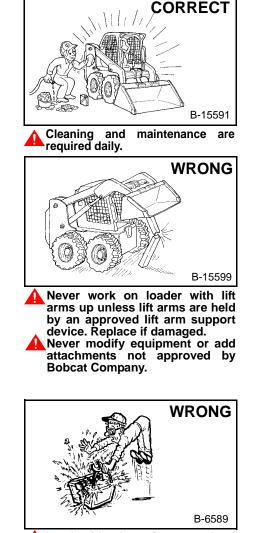
Lead-acid batteries produce flammable and explosive gases. Keep arcs, sparks, flames and lighted tobacco away from batteries.
