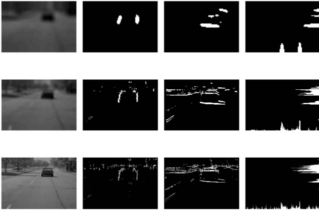
Fig. 5. Multiscale hypothesis generation—size of the images: 90 \times 62 (first row), 180 \times 124 (second row), and 360 \times 248 (third row). The images in the first column have been obtained by applying low pass filtering at different scales; second column: vertical edge maps; third column: horizontal edge maps; fourth column: vertical and horizontal profiles. All images have been scaled back to 360 \times 248 for illustration purposes (from [49]).
