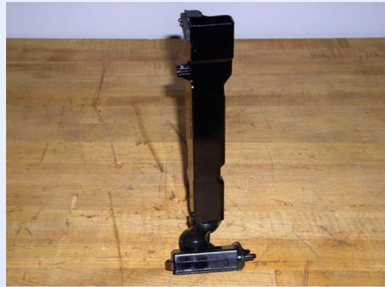
Fluid level control valve (outside transmission)
