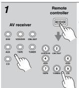
Use the AV receiver's input selector buttons to select the input source.
