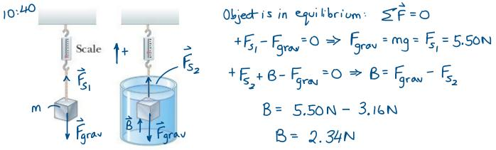
At the left, the figure shows a vertical spring scale. The top of the scale has a hook attached to the ceiling. The bottom of the scale has a hook attached to a rope. The rope hangs down and is attached to the object that hangs from the rope. At the right, the figure shows the same scale, but now the object is submerged in a tank of water. The reading on the scale at the right is less than the reading on the scale at the left. 2350 kg/m<sup>3</sup>
