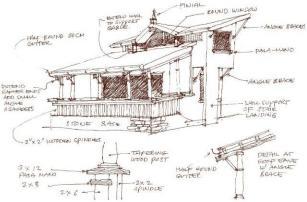
Figure 3: Tropical Design Features of Filipino Architecture
