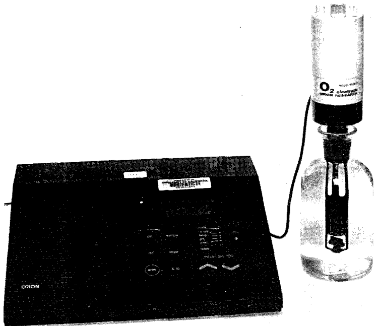
FIGURE 3-12 Measurement of oxygen in BOD bottle with a DO probe equipped with a stirring mechanism.
