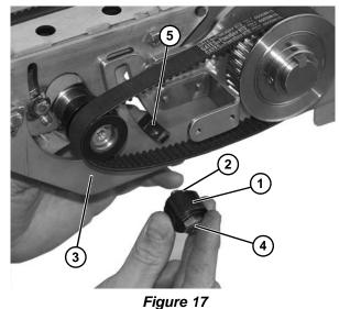
16. Using a straight edge, align driven pulley
