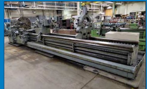
40" X 192" Monarch Model 3220-28-192 Geared Head Toolroom Engine Lathe
