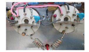
Two GY-50 wired in parallel are required for the power output specified.
