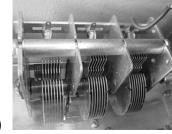
Note that the maximum capacitance is achieved when the plates are "meshed" together (a), that is, they are inter-laced. Minimum capacitance is achieved when the plates are "unmeshed" (b), that is, they are not inter-laced.
