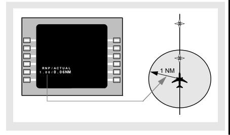
Oceanic RNPs are generally 4.0 or higher. Domestic en-route RNAV operations depend on the availability of radio updating (DME-DME) sources to support domestic RNPs. The following domestic RNP operations are fully supported by any Boeing FMC with DME-DME or GPS updating active:
