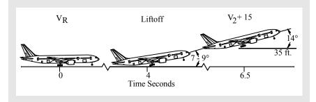
Retract the landing gear after a positive rate of climb is indicated on the altimeter. Retract flaps in accordance with the technique described in this chapter.
