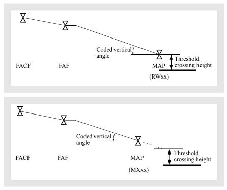
**Note:** The final approach course fix (FACF) is typically located on the final approach course approximately 7 NM before the FAF. The FAF referred to in the following procedures refers to the charted FAF and is intended to mean the point at which the final approach descent is begun.
