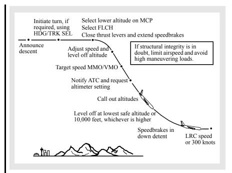
If the descent is performed because of a rapid loss of cabin pressure, crewmembers should place oxygen masks on and establish communication at the first indication of a loss of cabin pressurization. Verify cabin pressure is uncontrollable, and if so begin descent. If structural damage exists or is suspected, limit airspeed to current speed or less. Avoid high maneuvering loads.
