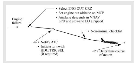
**Note:** If the airplane is at or below maximum engine out altitude when an engine becomes inoperative, select and execute the EO CRZ page and maintain engine out cruise speed.
