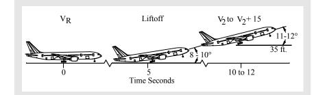
Retract the landing gear after a positive rate of climb is indicated on the altimeter. Retract flaps in accordance with the technique described in this chapter.
