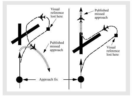
In the event that a missed approach must be accomplished from below the MDA(H), consideration should be given to selecting a flight path which assures safe obstacle clearance until reaching an appropriate altitude on the specified missed approach path.
