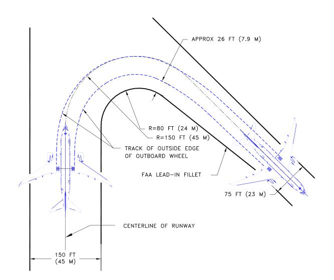
NOSE GEAR TRACKS CENTERLINE OF TURNS
