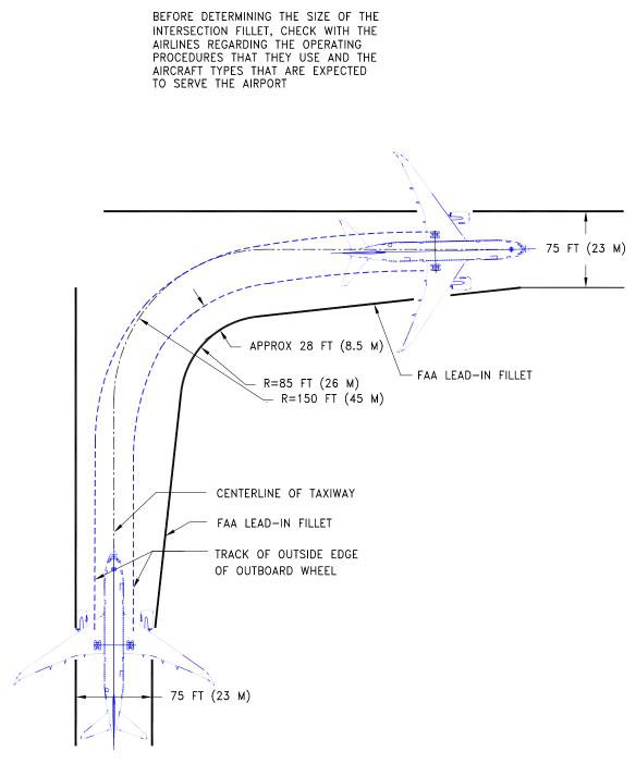
NOSE GEAR TRACKS CENTERLINE OF TURNS
