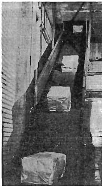
Reversible belt conveyor bringing supplement sections into mailing room for assembly with other sections of Sunday paper.
